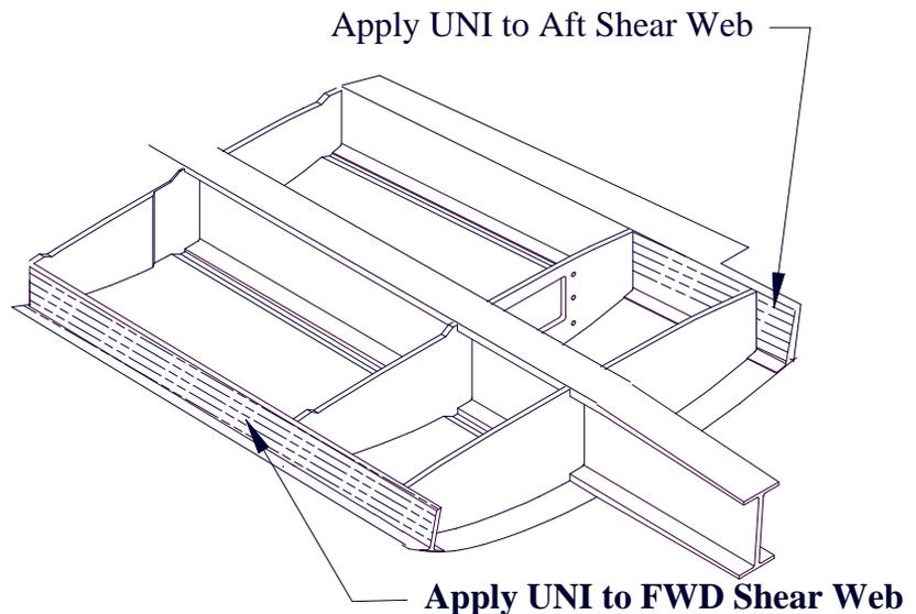
**Step 3 Apply Q-Cell Fillet and Fiberglass Tape.**
