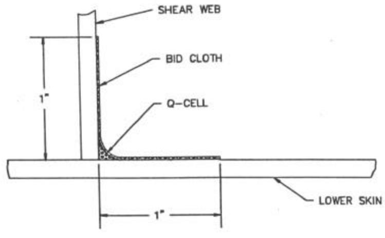
Mix resin to laminate the ribs and forward shear web.
