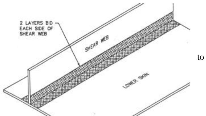
Remember to inspect all lay-ups for air bubbles and fit prior to the resin curing.
