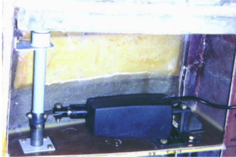
B. Drill the top 3/16" hole. Place a bolt through the bracket and the hole in the shear web. Clamp bracket in place, insure the bottom hole is centered on the vertical line and drill the bottom hole through the shear web.
