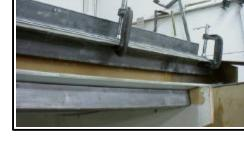
Recheck wing alignment and then place the load spreaders along the spar. Place the sand bags on the load spreader. Total weight along the main spar should total approximately 800 lbs. This weight should be distributed equally along the spar.
