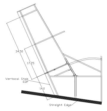
NOTE: If the hinges have already been installed on the rudder spar, insure that the spacing for the hinges match the vertical stabilizer.
