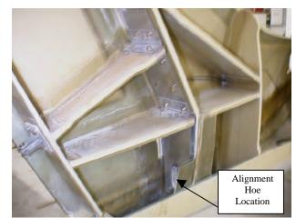
Make an alignment pin from a 3/16" bolt and screw it into the tapped hole. This pin should be no longer than 3/4".
