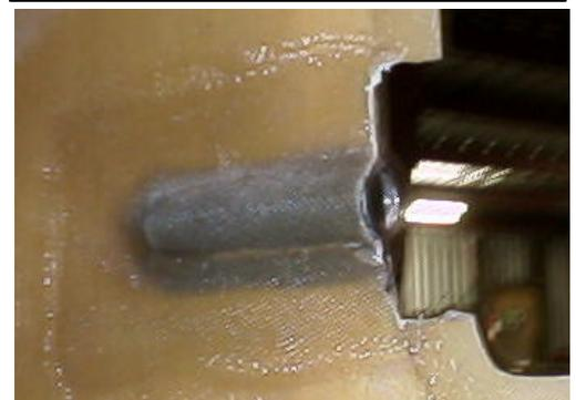
The tube will keep the receptacles parallel to the bottom of the door flange. Check to make sure you have maintained the 3" height above the bottom door joggle. Once you are sure of proper alignment use a milled fiber mix to secure in position. Position the receptacle so that the end can be ground off flush with the door jam.
