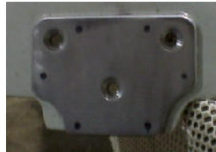
Turn the door over and countersink the fiberglass on the door to the normal countersink depth. Install the  $3/32$  rivet with the manufactured head on the fiberglass side. Buck the rivet so that the shop head fills the countersink on the aluminum doubler. Sand the excess rivet material off to a flush finish.
