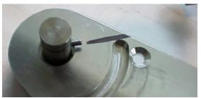
Temporally place the Inboard handle (**Single Pin Side Down**) on the pivot shaft. If the handle does not fit freely use a ream and clean out the pivot hole. Position the handle so that the pin fits in the machined grove the base plate. (Note: You may have to shorten the pin, or flatten one side of the pin so that it does not hit the side or the bottom of the grove when the handle is snug against the bushing flange.
