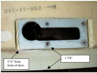
the door. (Note: Make sure the bottom edge of the door has been it to the fuselage.) Mill Fiber the G10 block in place. When cured cut out the inner area so that the base plate can be inserted into the G10 mounting block. The outer flange of the base plate should be flush with the outer door skin. If not sand the G10 block to achieve this fit. When installing the G10 Block in the Baggage Door, center the block fore and aft.
