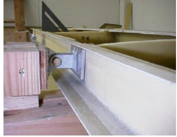
D. Bond the aft shear web to the lower skin using a milled fiber / resin solution.
