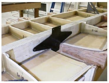
F. Install AN3-10A bolts and washers. Torque all bolts & screws to 20-25 inch pounds.
