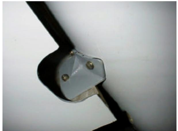
**Step 8. Final drill / ream the 8 spar pin holes and install spar pins.**
