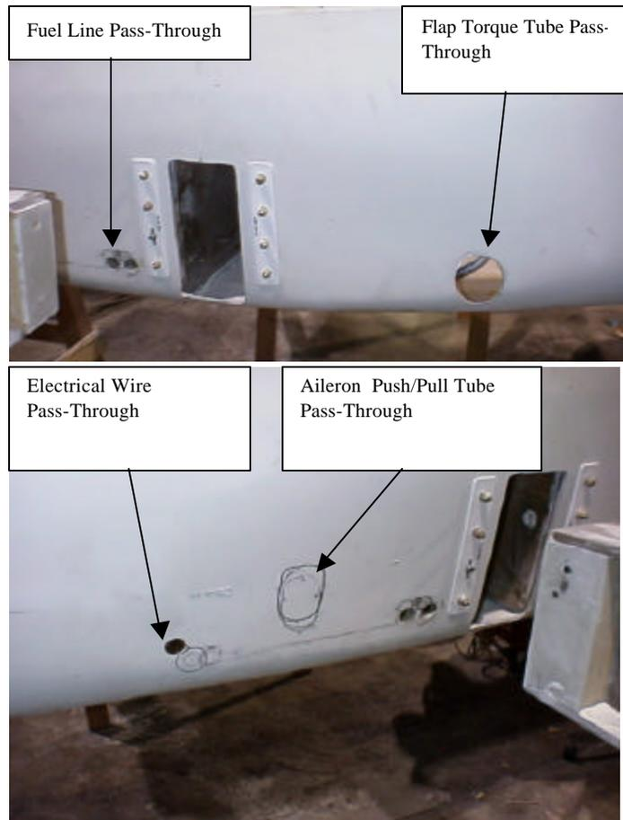
Slide the wing into the fuselage and install the upper inboard temporary pin partially into the wing spar to hold the inboard end into position. These temporary pins are not supplied in the kit. We recommend that you use 7/16" drill rod purchased from your local hardware store. (Note: You may need to remove some of the material on the aft leg of the forward attach bracket in order to allow it to slip far enough onto the forward shear web.)
