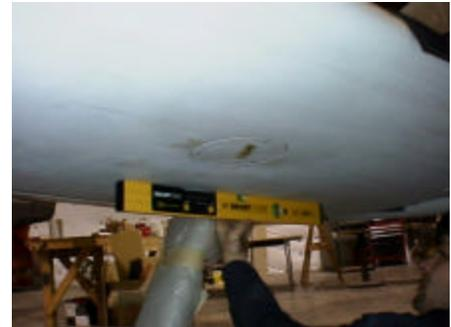
Set the wing template at the WBL 36 scribe line and set the wing at 1.5 degrees of positive incidents.
