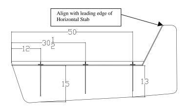
glue in place. Drill the holes for the mounting bolts and secure the hinge to the elevator spar. (Note: Use non-aviation nuts to secure the hinges. Once the spar is attached to the skin the hinges will be removed and anchor nuts will replace the nut for final assembly.
