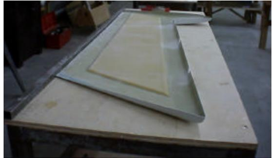
**Step 2. Locate Rudder Hinge Mounting Points on Spar.**
