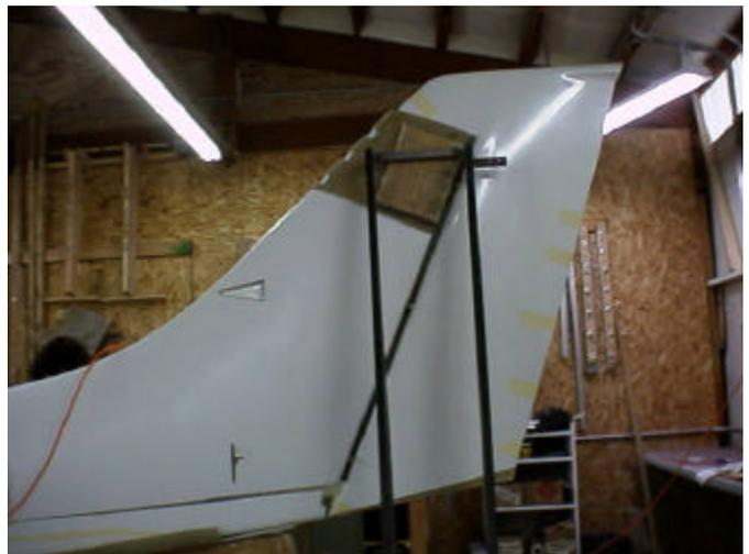
**Step 6. Install Rudder Ribs.**
