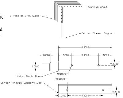
Place the center nylon blocks on the torque tube assembly and bolt the aluminum angle to the blocks using AN 3-21A bolts. **Do not tighten the bolts at this time.**
