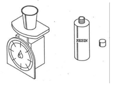
Using a syringe marked in .10 cc increments, carefully measure the amount of catalyst, and gently squirt it into the mixing cup. Immerse only the tip of the syringe, not the barrel. Use a wooden tongue depressor with one end cut square to stir the resin. This allows you to scrape the corners of the cup.
