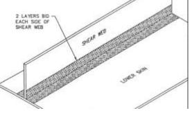
Apply the resin with the brush being careful not to put too much resin on, because excess resin is difficult to remove.
