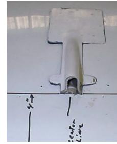
Laminate 6 plies over the cut out area on the inner side of the elevator skin to form the access panel joggle. This laminate should extend onto the elevator skin at least 2". When cured remove the access panel and trim the inner area so that you have a ½ inch joggle around the left, right and front sides of the panel.
