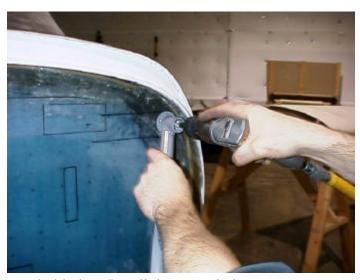
boltholes as drill guides and drill the two upper boltholes. Install the upper bolts.
