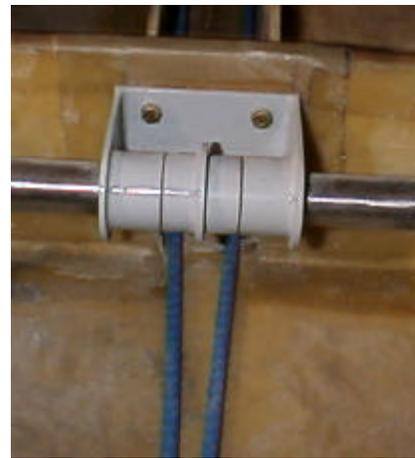
**Recommended Rudder Cable Placement.****Step 3. Install aft Rudder Bellcrank.**
