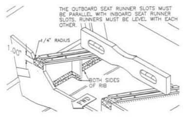
Seal all of the exposed foam along the upper edges of the forward shear tie and seat gusset with one ply of bid cloth.
