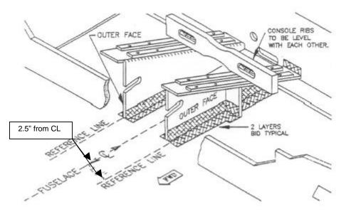
are aligned level with each other. The slots must be parallel with each other and 90° to the carrythrough. Prep the area. File and fit at all mating surfaces and hot glue in place. Apply Q-cell fillet and two layers of bid cloth to the joints.
