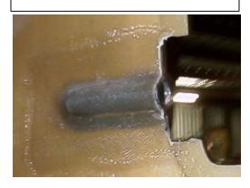
The tube will keep the receptacles parallel to the bottom of the door flange. Check to make sure you have maintained the 3" height above the bottom door joggle. Once you are sure of proper alignment use a milled fiber mix to secure in position. Position the receptacle so that the end can be ground off flush with the door jam.
