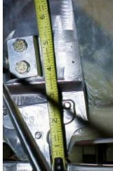
When cured, place the Cabin Door Strut Mount Bracket (with the beveled edge forward) in the center of the hardpoint and locate the two 5/15 holes. Drill these holes and install 5/16–24 helicoles into the holes. Use caution not to drill through the door skin.
