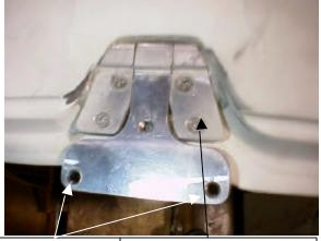
Place straight edge from front and rear hinge aligned with these two holes
