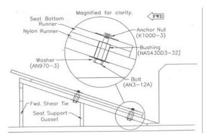
Move the seat bottom runners to their full aft position. Put the seat on the runners with its back against a 0.5" spacer temporarily taped to the spar carry-thru. Leave 0.5" clearance between the seat and the fuselage wall. On the edges of the seat bottom runners, mark the points of contact between the anchor nuts and the seat bottom. Also draw marks on the seat bottom, showing the position of the runner. Take the seat out.
