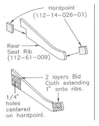
The rear seat ribs (112-61-009) are placed between the floor-mounted fuseslage ribs for the right and left rear seats.
