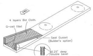
With a hole saw, motto-tool, or sandpaper, remove enough of the seat bottom to clear the anchor nut for 0.5" around each mark (see Fig. 5.150-4). Apply a layer of milled fiber on the seat bottom runners where they contact the seat.
