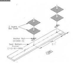
Cut eight 2.0" square pieces of bid cloth. Punch a hole through the center of each square with a hole punch for bolt openings. Apply milled fiber to the anchor nuts, avoiding the threads. Laminate two pieces of bid cloth over each anchor nut, centering the holes over the boltholes. Allow it to cure.
