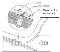
Place the seat, within the reference marks drawn earlier, with the seat back resting against the 0.5" spacer. Weight the seat so that it presses tightly on the runners, and let the mixture cure undisturbed.
