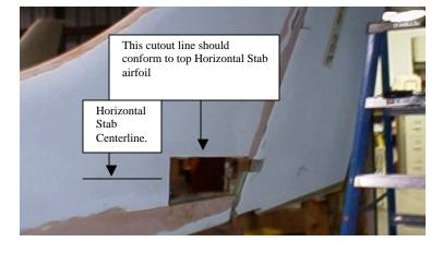
bulkhead 235, level with the horizontal stab alignment hole. Drill a 1/8" hole through the left empennage skin. The horizontal stab is set at 0° incidents so use a level and draw the horizontal stab centerline on the left outside empennage skin.
