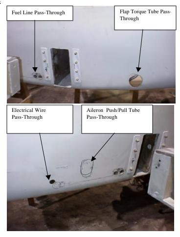
Slide the wing into the fuselage and install the upper inboard temporary pin partially into the wing spar to hold the inboard end into position. These temporary pins are not supplied in the kit. We recommend that you use 7/16" drill rod purchased from you local hardware store. (Note: You may need to remove some of the material on the aft leg of the forward attach bracket in order to allow it to slip far enough onto the forward shear web.)
