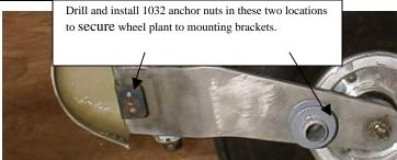
Remove the wheel pant and install 10-32 anchor nuts to the four attach point holes. Install 8-32 anchor nuts to the wheel pant flange. Reinstall the wheel pant to the nose gear yoke.
