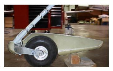
Step 4. Attach Wheel Pant to Front and Rear Bracket.
