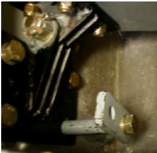
Inboard bracket with flat actuator bracket installed
