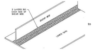
onto the wing skin. Wet out the cloth using the resin and a brush. Remove any bubbles before going on to the next ply. Apply the second ply over the first one and wet it out. After both plies are laid up and wet out, remove any bubbles and excess resin using a brush or squeegee. Do this to all ribs and shear webs.
