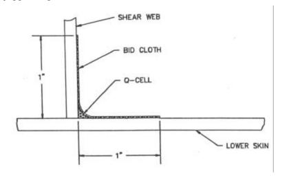
Mix resin to laminate the ribs and forward shear web.
