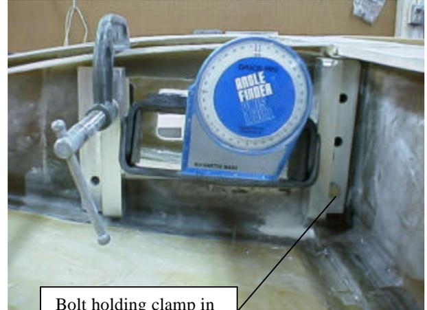
Bolt holding clamp in position in # 3 hole.
