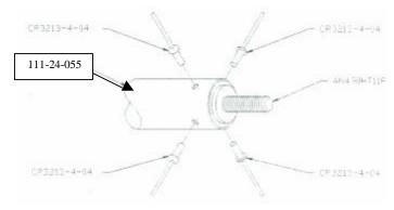
the spacer and rod end to the other end of the tube in the same manner.
