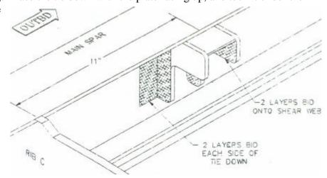
onto both ribs and the shear web. The tie down hole will be drilled in the wing closeout section.
