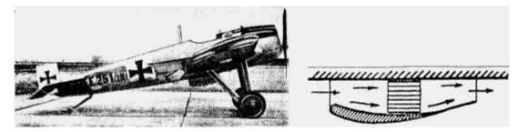
Towards the end of W.W. 2, the ringradiator was extensively used by the Germans because relative lightweight armourment could protect the segmented cooling system. The close proximity to the propeller and the relative thick propeller section could slow the inflowing air down by 20 percent, but a large spinner
