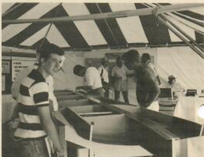
Wing Kit with ribs, shearweb and hardware installed on display.
